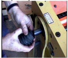
3. Remove the top cover/collector shield and the handle. (whether you have the side or top mounted handle, the key will usually fall free)
