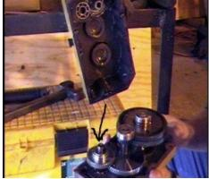
19. Remove the bolt inside the helical gear and remove them both.
