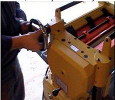
4. Before removing the side gear cover, remove the guard located on it's back side at each lover corner.
