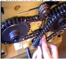
6. Remove the three bolts from the gears to expose the keys. It should be possible to rotate the cutter head enough to align the keys in an upward position.
