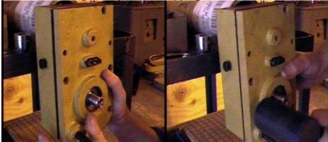
29. Tighten all of the screws in an alternating sequence.
