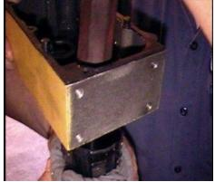
26. Start the journal end through the back of the bearing, using a socket against the face of the bearing, ensuring it only makes contact with the inner or outer race and not the rubber seal, the use of a washer with the same ID and OD of the bearing is recommended to protect the seal. The end of the bearing and Journal should be flush.
