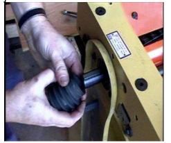
36 The protective wrap can now be removed by slitting it longways between two rows of knives. Rotate the head while rolling off the wrap.
