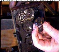
20. Before driving the cutterhead from the bearing and housing, reinsert a spare M6 screw back into the journal end. If you use the original screw, it will probably be damaged.
