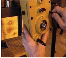
30. Refill the gearbox with the 50 weight oil that was removed.
