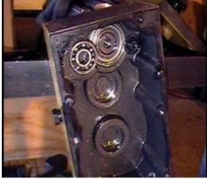
24. At this time, install the bearing on the pulley end of the new head (snug press fit). The pulley can be used to seat the bearing. With the outside of the pulley (large OD) against the bearing, tap it into place.
