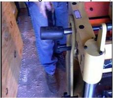
12. Remove the head and gearbox together.
