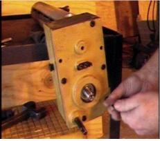
15. Drain the gear oil into a clean container.
